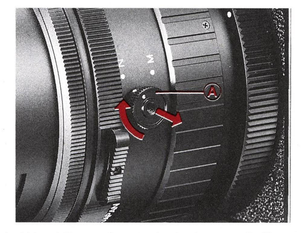
1. Pull out the mirror release knob (A) while turning it clockwise, and align the red dot on the knob with the mirror up indicator (M).
