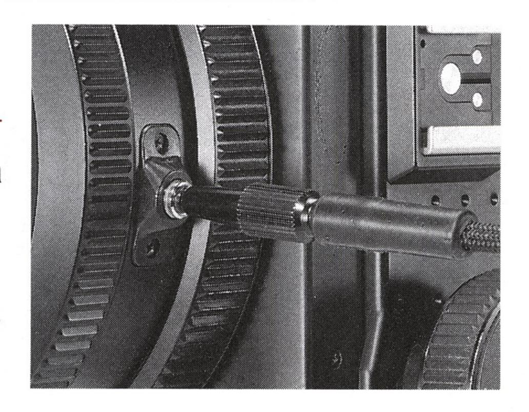
1. Screw the black tipped cable release into the mirror-up socket until it is snug, and the release socket will then elevate. Then screw the chromium-tipped cable release into the shutter release button on the side of the body.
